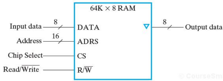
Symbol for a 64\text{K} \times 8 RAM Chip
